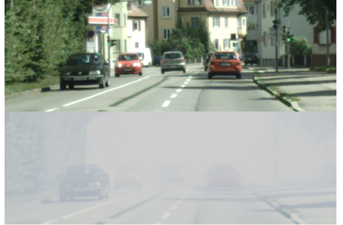
Fig. 4. The upper image is from the Cityscapes image data set, the lower figure shows that image with our fog applied. Distant objects are harder to spot than closer ones, as they are affected more by the fog.
