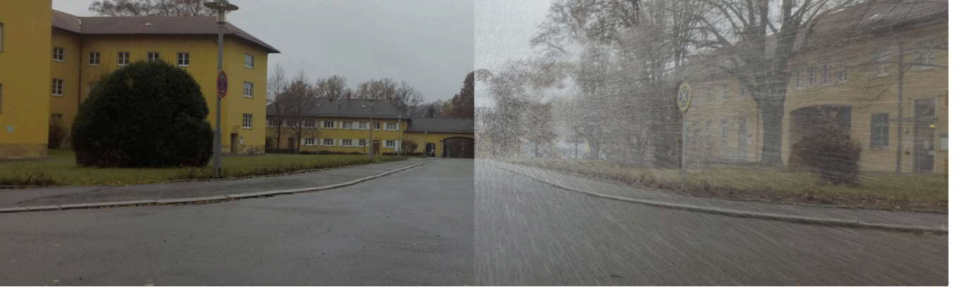
Fig. 1. Example of a street image before and after augmentation with both snow and fog. On the left half the image is shown unaltered, on the right side we simulated falling snow at a vehicle speed of 50 \text{ kmh}^{-1} , a snow fall speed of 1 \text{ ms}^{-1} and crosswinds of 1 \text{ ms}^{-1} as well as light fog with the method proposed in this paper. Motion blur is visible especially towards the edges of the scene. Image depth was calculated from a pair of stereo images.
