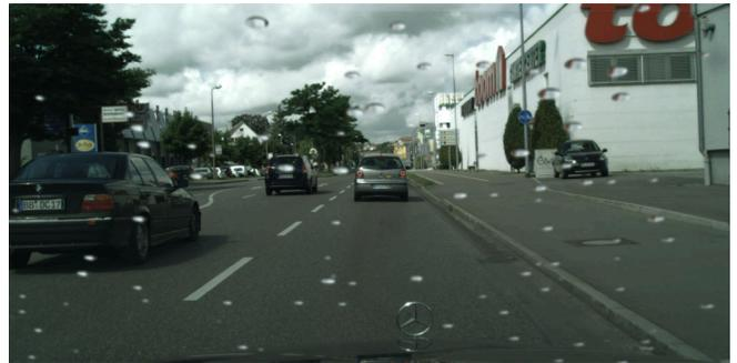
Fig. 5. Example image from the Cityscapes data set with rendered raindrops. The windshield was placed 30 cm in front of the camera and tilted to  $27^\circ$  from the horizontal. The drop radii have their mean at  $\bar{r} = 1.5$  mm and a standard deviation of  $\sigma = 0.4$  mm. The raindrops were convoluted with a disk kernel to simulate out of focus effects [33].
