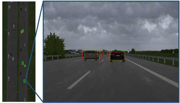
Fig. 4. Snapshot of the simulated highway scenario. The left image shows the birds-eye-view of the ego vehicle's environment and the right image presents the camera sensor view of the ego vehicle. The red and green boxes indicate the local and the collective perception, respectively.
