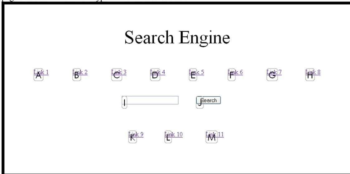
**Figure 1.** *The Nessi Browser screen during tag presentation. A letter corresponding to the P300 spelling matrix is assigned to each hyperlink, to indicate to the users which letter they have to chose from the matrix to select a hyperlink.*
