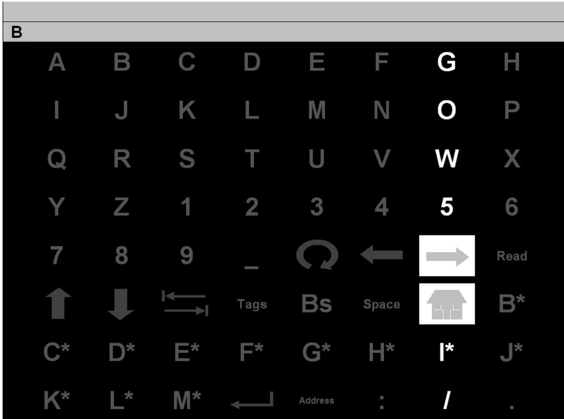
**Figure 2.** The Nessi matrix screen, with all icons represented. Characters and symbols are highlighted in rows and in columns. Above, an example of a highlighted column; for icons, the colors invert. Also, feedback representing what is typed is shown; here, it is the letter “B”.
